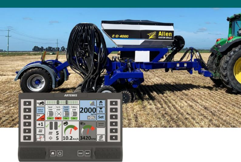
The new generation RDS Artemis drill control system is a variable rate control and monitoring system for seed drills. The system removes the need for a mechanically driven landwheel by operating the metering unit with an electric motor maintaining its speed proportional to forward speed, or adjusting sowing rates to suit the mapping provided by the precision farming option if this is utilised.
